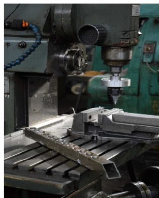
Fig. 4. Milling machine with mounted thermal drilling set.
